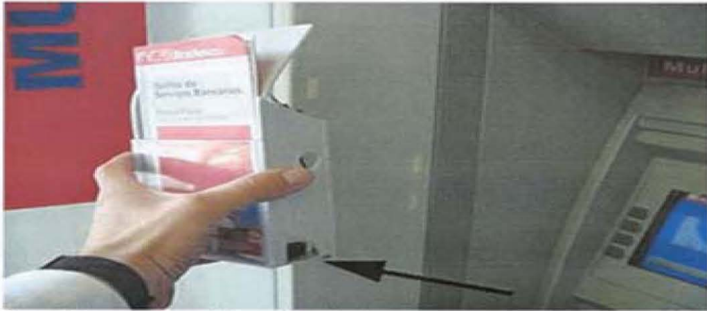
The PIN reading camera being installed on the ATM is housed in an innocent looking leaflet enclosure.
